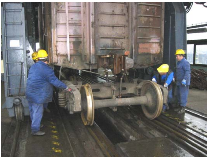
Figure 1 Treating interoperability discontinuity. Exchange of axles in Záhony
